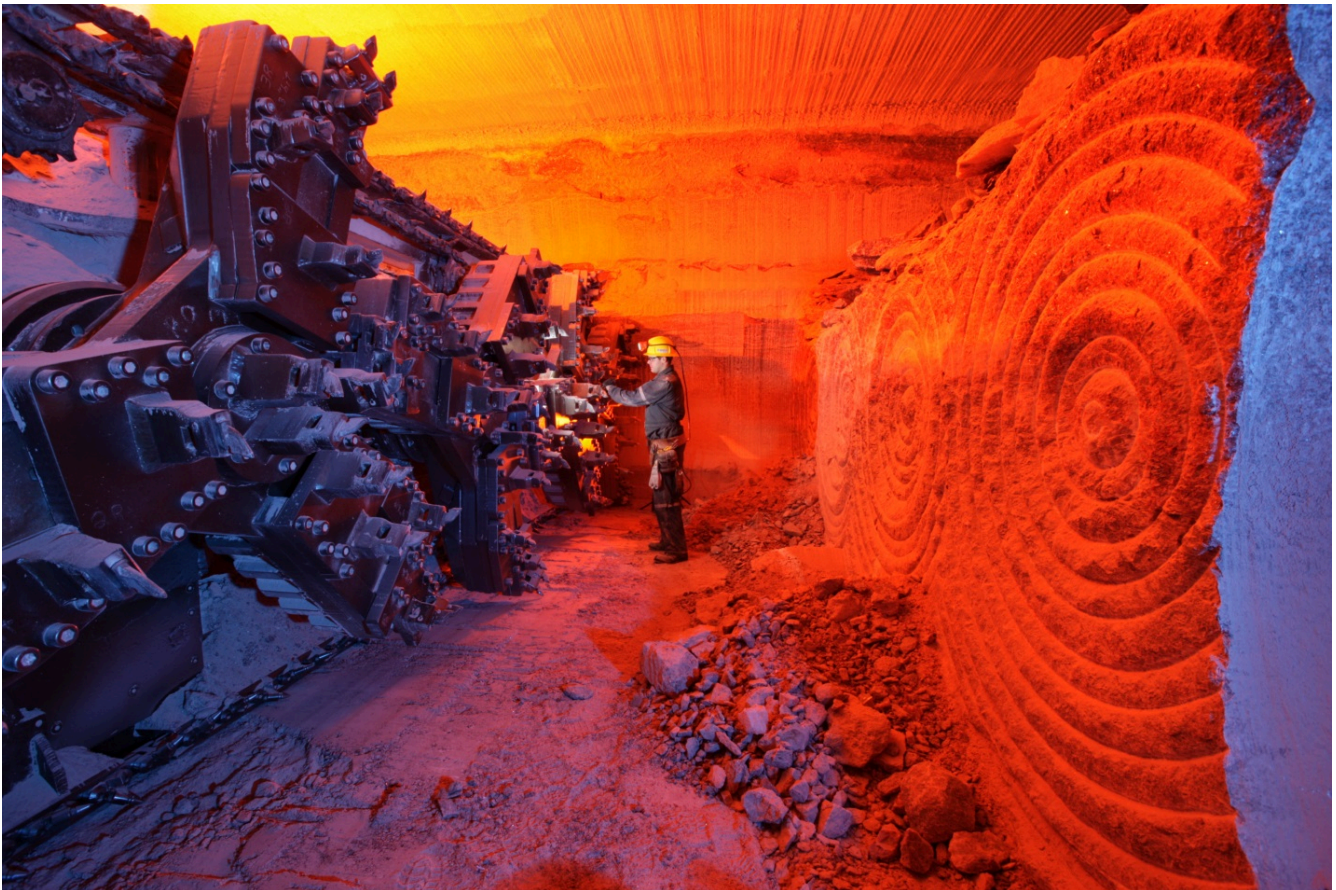
Figure 6.2.8 A mining machine at the face of potash ore (sylvite) in the Lanigan Mine near Saskatoon, Saskatchewan. The mineable potash layer (on the right) is about 3 metres thick.
