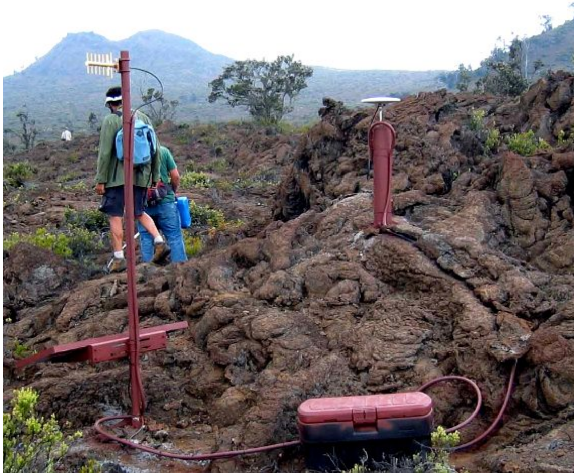
Figure 4.5.2 A GPS unit installed at Hualalai volcano, Hawaii. The dish-shaped antenna on the right is the GPS receiver. The antenna on the left is for communication with a base station.
