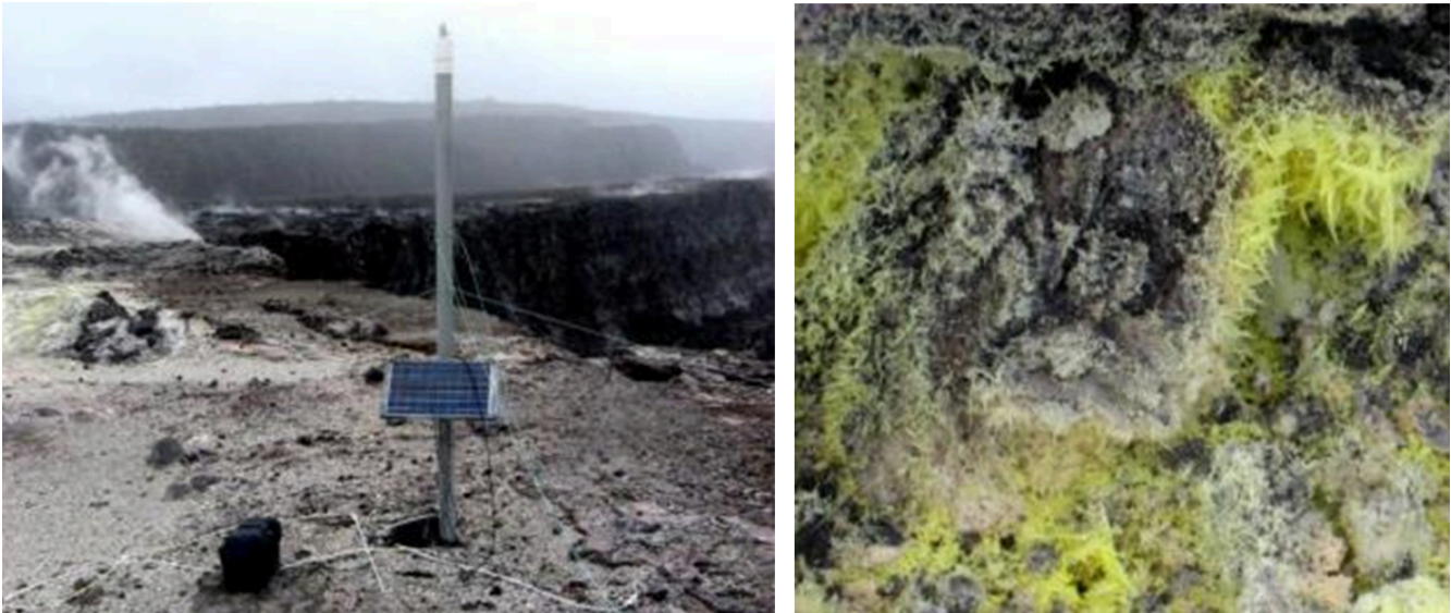
Figure 4.3.10 A gas-composition monitoring station (left) within the Kilauea caldera close to the edge of Halema'uma'u crater. The rising clouds are mostly composed of water vapour, but also include carbon dioxide and sulphur dioxide. Sulphur crystals (right) have formed around a gas vent in the caldera.
