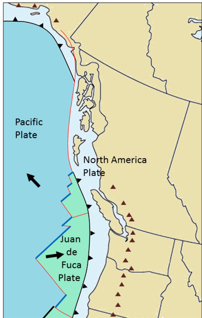
Figure 21.5.4 The current plate situation along the western edge of northern North America. Blue lines are divergent boundaries, red lines are transform boundaries, and black lines with teeth are subduction boundaries. The dark red triangles are volcanoes. [Image Description]
