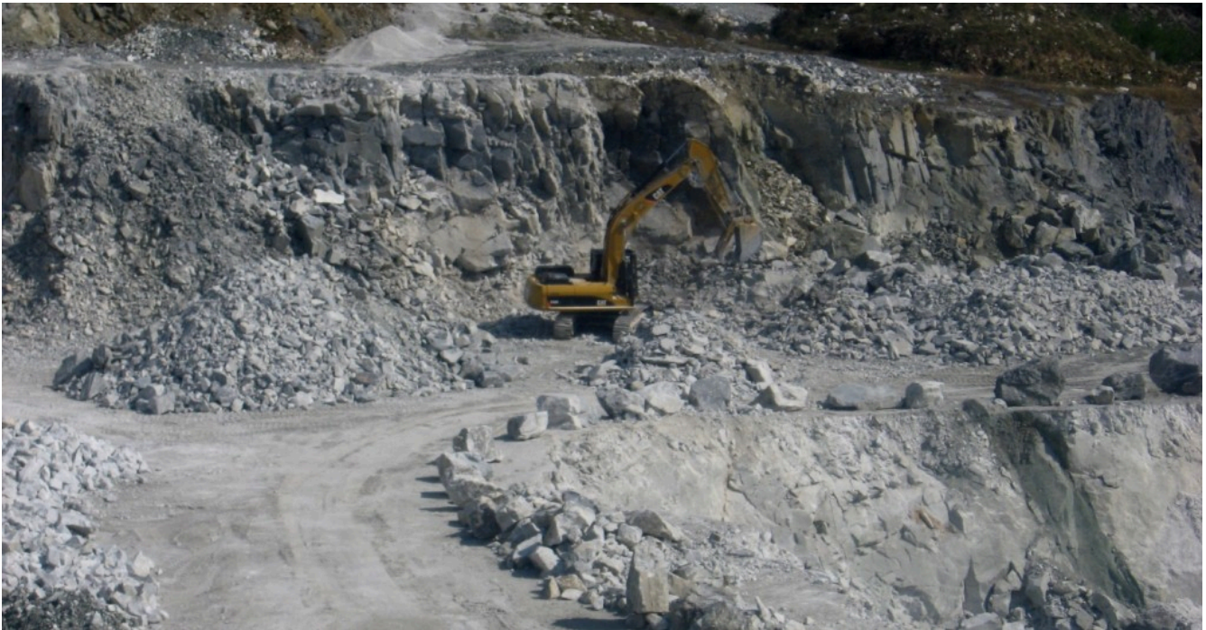
Figure 20.2.2 Triassic Quatsino Formation limestone being quarried on Texada Island, B.C.
