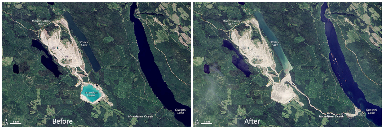
Figure 20.1.11 The Mt. Polley Mine area before and after to the dam breach of August 2014. The tailings were stored in the area labelled “retention basin.” The retention dam failed and water and tailings released flowed into Polley Lake, Hazeltine Creek, and Quesnel Lakes.
