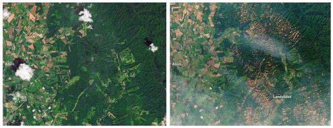
*Figure 15.1.7 Slope failures in the Sapporo area of Japan following a typhoon (Sept. 4th, 2018) and earthquake (Sept. 6th, 2018) (Before and after Landsat 8 images: left: July 2017, right: September 2018).*
