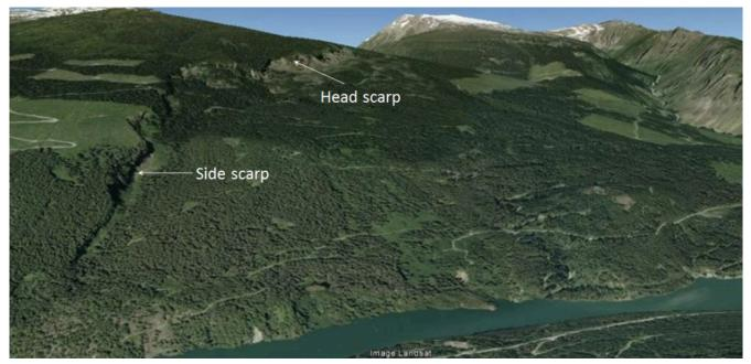
Figure 15.2.3 The Downie Slide, a sackung, on the shore of the Revelstoke Reservoir (above the Revelstoke Dam). The head scarp is visible at the top and a side-scarp along the left side.
