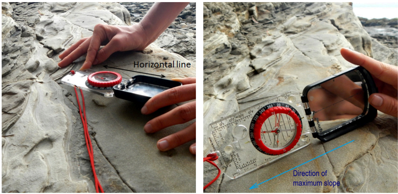
Figure 12.4.2 Measuring the compass direction of the strike (left) and the vertical angle of the dip (right) using a compass with a clinometer.
